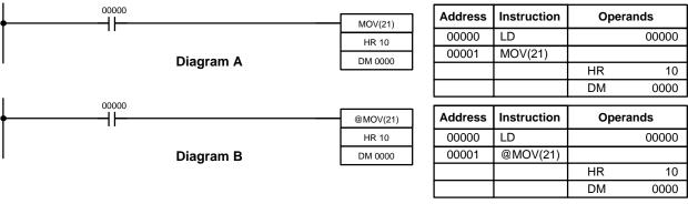
In diagram A, the non-differentiated MOV(21) will move the content of HR 10 to DM 0000 whenever it is cycled with 00000. If the cycle time is 80 ms and 00000 remains ON for 2.0 seconds, this move operation will be performed 25 times and only the last value moved to DM 0000 will be preserved there.
